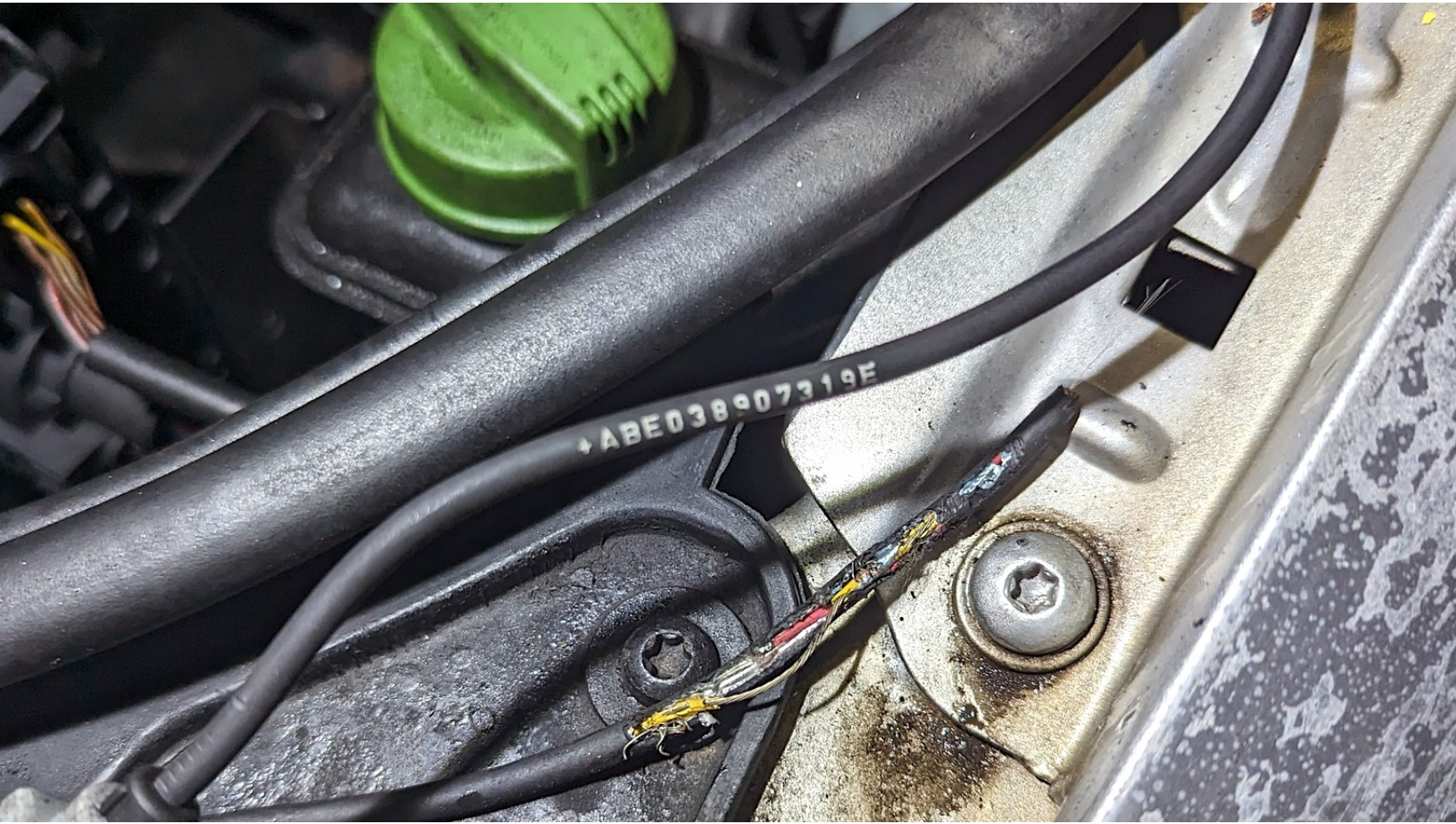
Sensor wiring chewed by a rat. Image: RAC
